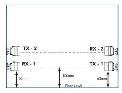
e. ATA recommends the transmitter and receiver are placed in line of sight, with the beam 100mm above the ground level (as per AS60335). This can be achieved by ensuring the bottom of the receiver and transmitter are 65mm above ground level. They should also be placed as close as possible to the door / gate opening.In industrial applications it is recommended that multiple Safety Beams are fitted.
