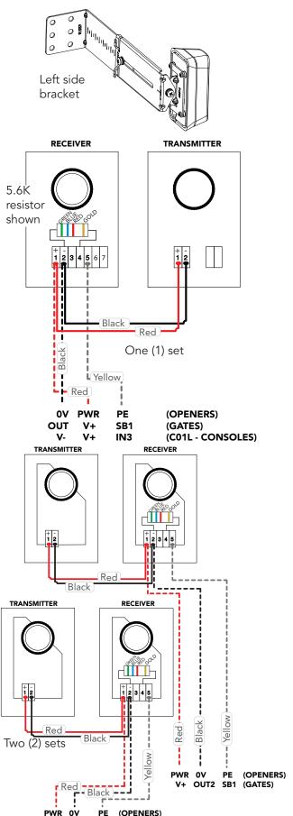
**NOTE:** Mount the receiver on the side of the doorway / gateway closest to the opener / console.
