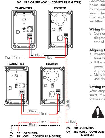
NOTE: Mount the receiver on the side of the doorway / gateway closest to the opener / console.
