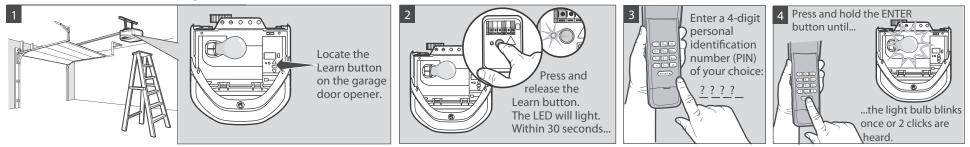
To test, press the PIN, then press the ENTER button. The garage door opener will activate. To program the Wireless Entry Keypad to more than one garage door opener, repeat the steps above using a new PIN for each additional garage door opener.
