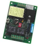
2-Channel 27MHz GIGALINK™ Receiver with relay outputs, GLR2702
