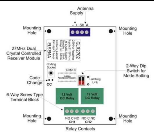
Sh terminal is used for antenna's using coaxial cables. The shield (braid) on the coaxial cable should be connected to the Sh terminal while the core of the coaxial cable is connected to the A terminal.
